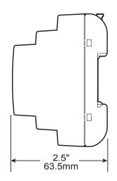
The U60 modules are designed for DIN-rail mounting; dimensions for both modules are the same
